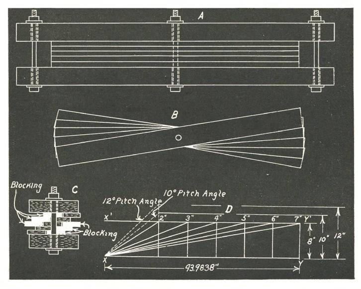
well. Place one section of the yardstick over the center bolt on the bottom half of the clamp, and coat with glue, adding one section at a time, being sure the glue is well spread between the surfaces by gently working each layer on the one next beneath. When all five layers are glued, spread fan-wise the ends of the sections, each section allowing half of the one beneath to show at the end. See illustration (B). Put on the top half of the clamp, setting up the center bolt only.
