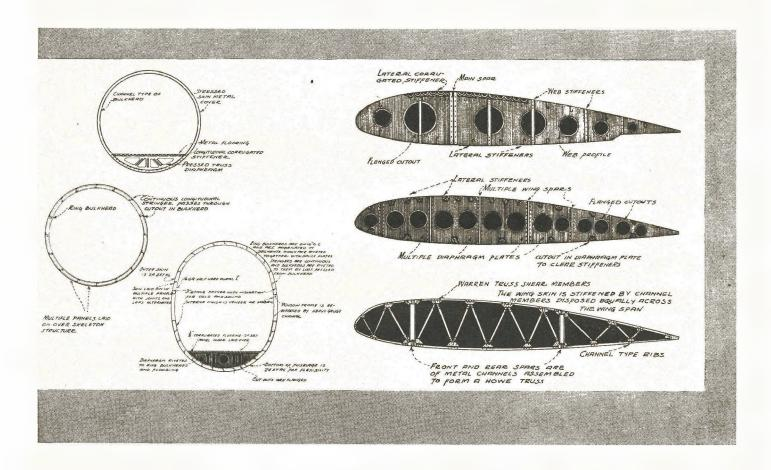
Far left—How Ryan builds their metal fuselages. Their method features a heavy skin that carries most of the load. Left in the photo is shown the tail section of the S-C, center, the fuselage center section and, right, the cabin section still in its jig. The drawings show, left, the three basic methods of stiffening a thin-
