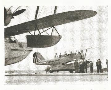
Seen from beneath the lower wing of the giant Hall-Aluminum is a Grumman JF-2 four-place amphibian. This smaller type of plane is similar to the Navy JFs, and is intended for patrolling only.
