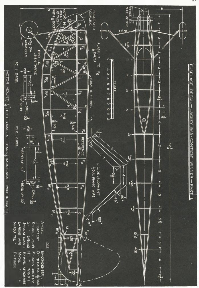
cement is drying. Check the sides with a square to see that they are at right angles to the working surface. Cement in the remaining cross pieces, with the landing-gear assembly taking the place of balsa pieces at those positions. The landing-gear joints at the wheels may be bound with tinned wire and soldered.
