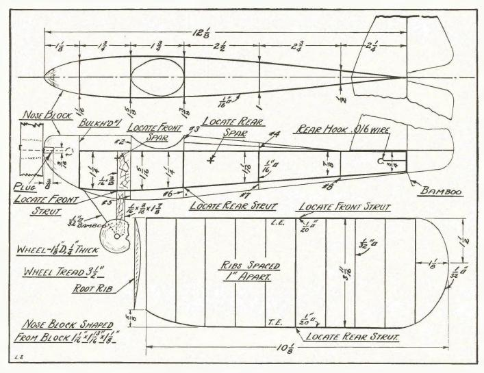
A novel construction feature in the by form of an indoor flying scale model. LAWRENCE SMITHLINE
