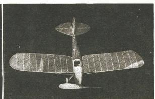
Much pleasure can be derived from an indoor flying scale model. The Heath Midwing proved itself an excellent flier, stable and reliable. The two characteristic poses—right—show the pertinent assembly details and the opaqueness of the microfilm-covered wing and tail. Fuselage is covered with superfine. This ship is capable of nearly four minutes' duration.
