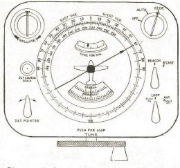
Diagramatic drawing of the face of the "pigeon." The crank at bottom revolves the inner dial band.
